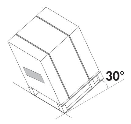
• Insert the forks from the side so as not to damage the panels.
