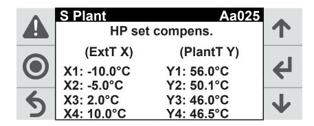
This menu can be used to set the heating curves for winter operation.
